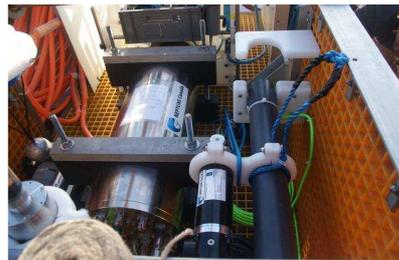
*Junction Box installed on Deployment Rig (Credit: Venus)*
